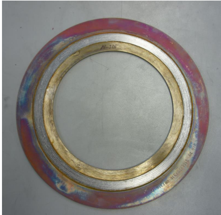
Fire test according to API 6FB (MESC SPE 85/300 - 3.3.3) – 14-326
