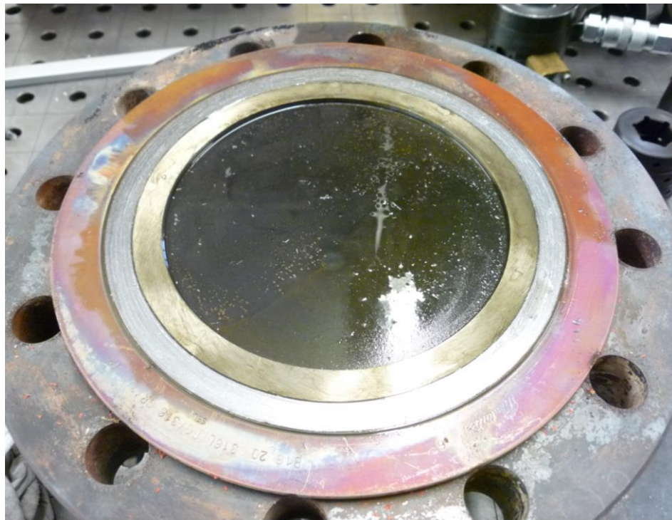
Fire test according to API 6FB (MESC SPE 85/300 - 3.3.3) – 14-326
