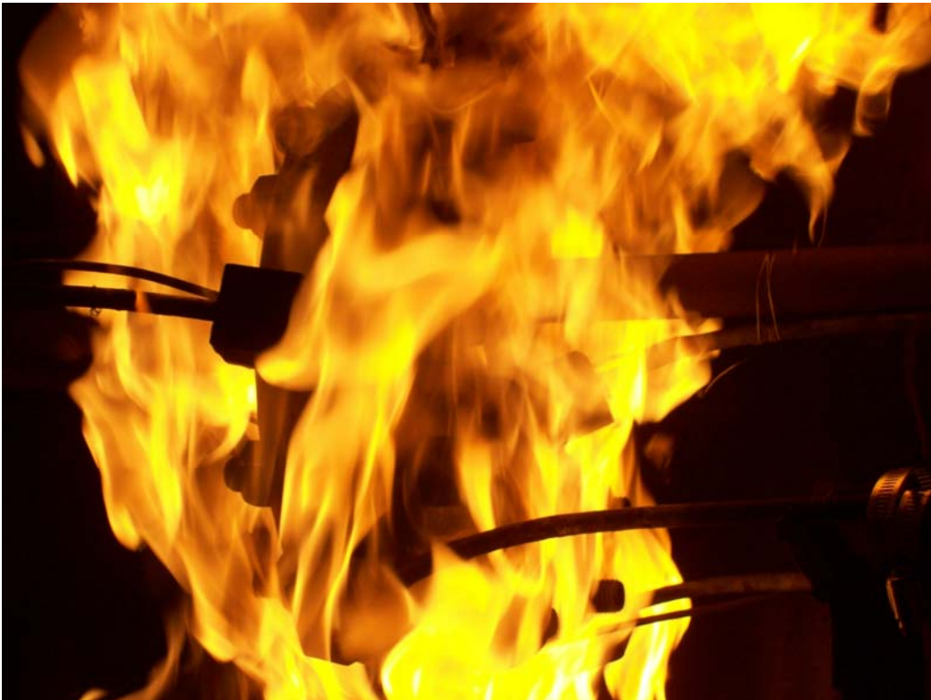
Gasket Fire Test
