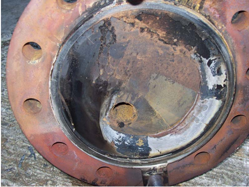
Gasket After Test
